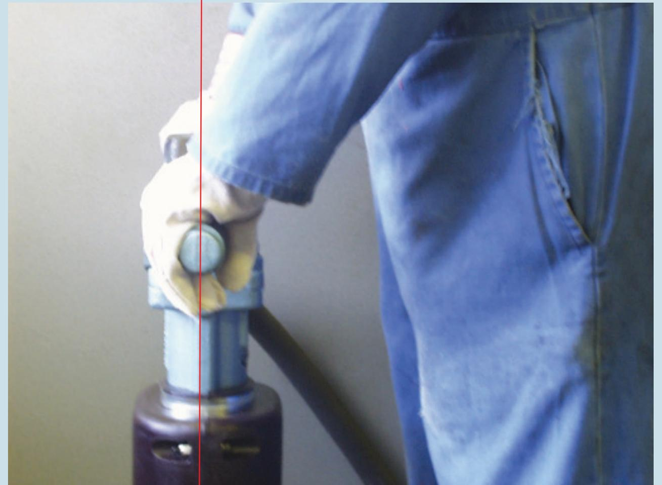
*Try to keep the breaker as near vertical as possible during operation.*
